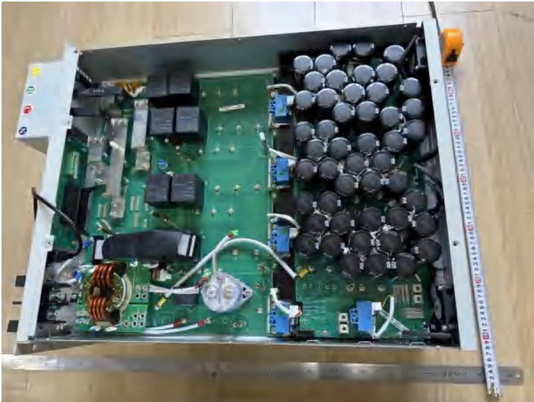
Figure 9 Inside view without control board, isolation board
