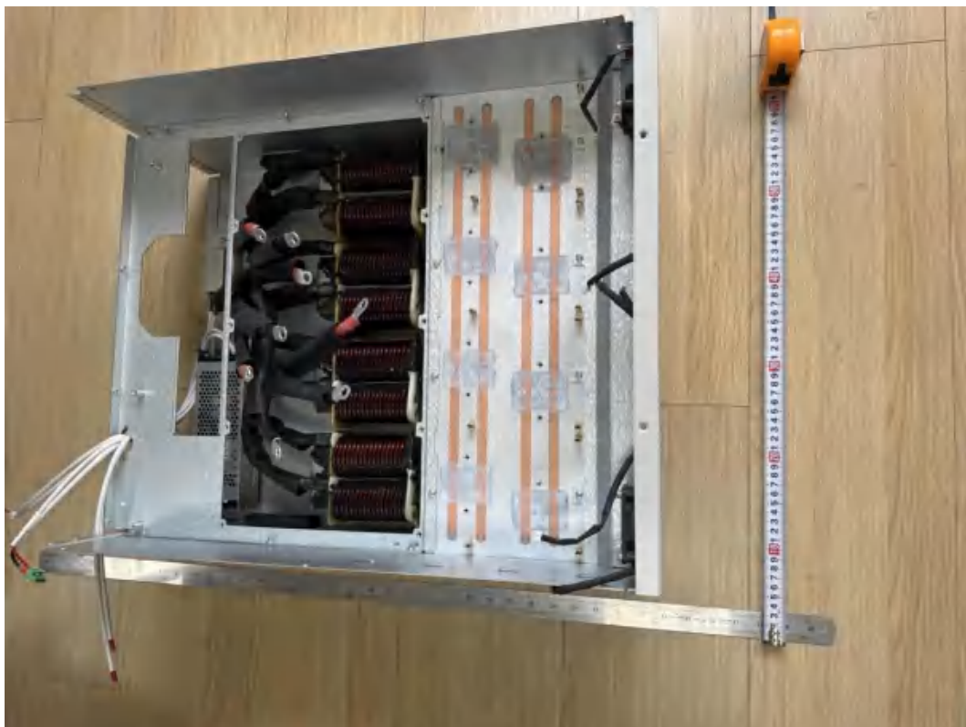
Figure 12 Inside view of enclosure without PCBs
